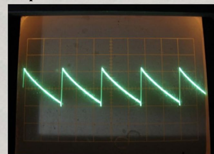
Output Is Inverted Sawtooth Waveform
